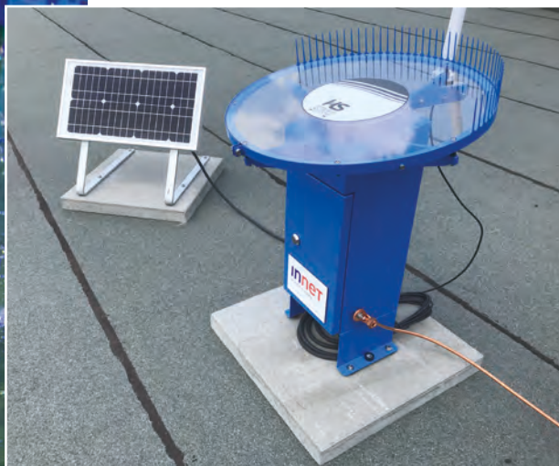
Figure 2: HailSens Model R&D/INS: Swiss HailSensor Network – typical flat roof installation. Image: inNET Monitoring
